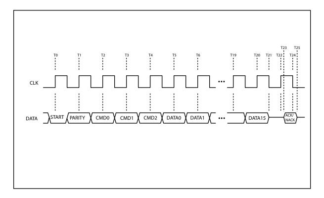
T0 marks the start of the transaction. DATA IO is driven low indicating a start-bit.
