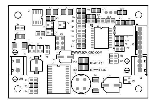
**D1** Reverse Polarity Protection Diode
