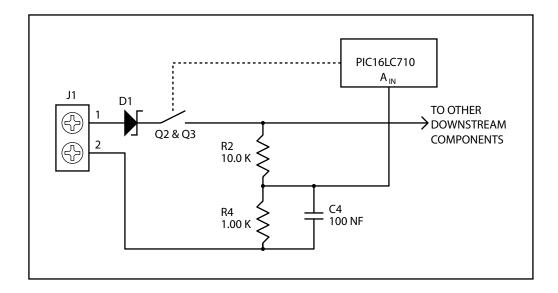
The voltage divider composed of R2 and R4 is placed after the downstream control switch (Q2 & Q3). This means that a low voltage test may only occur when Q2 & Q3 are "closed." This was done to save power when downstream devices are de-energized.
