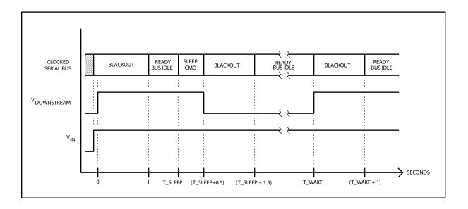
Just prior to 0 seconds, Vin comes up. This resets the PowerNut's processor and very shortly thereafter, the downstream connector is energized. At the 0 second mark in the figure, downstream power is turned on and a 1 second communications blackout starts. At the 1 second mark the PowerNut will accept commands on the clocked serial bus.
