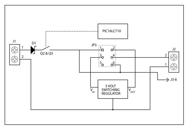
To configure the downstream voltage on J2 to be 5 volts, JP3-1 and JP3-3 must be shorted along with JP3-2 and JP3-4.
