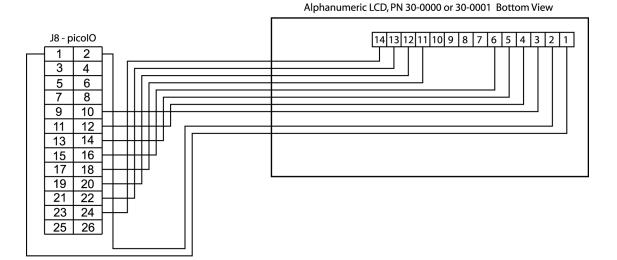
The following chart details the cable pinout and signal names used for connecting an LCD to the picoIO. The signal names are given for information only and are not needed for normal operation of the LCD.
