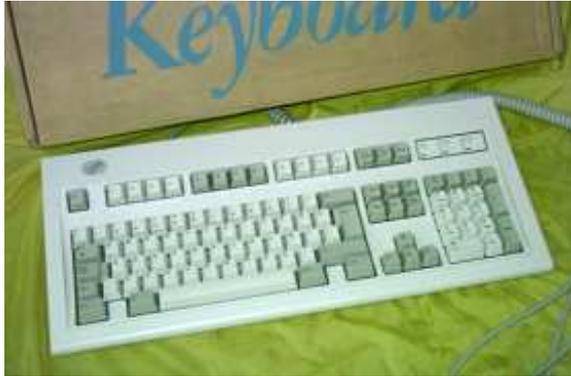
The keyboards have always been the most favorite units for data input to the computers. The PC AT keyboard has not changed electronically and protocol-wise since the announcement of the first IBM PC AT in 1984. It has evolved into its current layout and connector with IBM PS/2 series in 1987, and thus has been started to be called as the **PS/2 Keyboard**.
