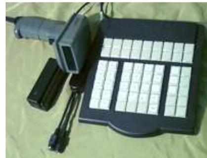
If one takes a close look at PS/2 keyboards; it will be seen that they consist of matrix keypads (whose size has grown up to 8 rows by 16 columns) and a controller (such as Intel 8048) which encodes the row-column information. Our PCs have a complimentary controller (such as Intel 8042), which acts as a 'host' and decodes this information. An embedded system targeted for PS/2 connectivity should realize the functions of this decoder.
