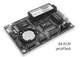
On a form factor slightly larger than a credit card, we've implemented a 40MHz x86 DOS computer. The system features ½ megabyte each of RAM and Flash memory, two serial ports, battery-backed clock calendar, 10Base-T Ethernet and a socket for optional M-Systems DiskOnChip products. Also included on the board are 16 bits of digital I/O, a watchdog timer, RS-485 and TTL serial port I/O, and LCD and keypad drivers.
